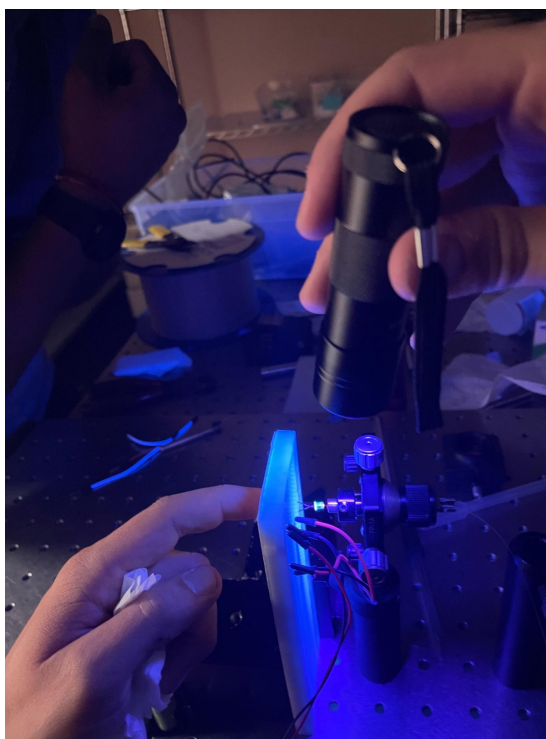
Figure 6.1-4. UV Flashlight Curing UV Resin
