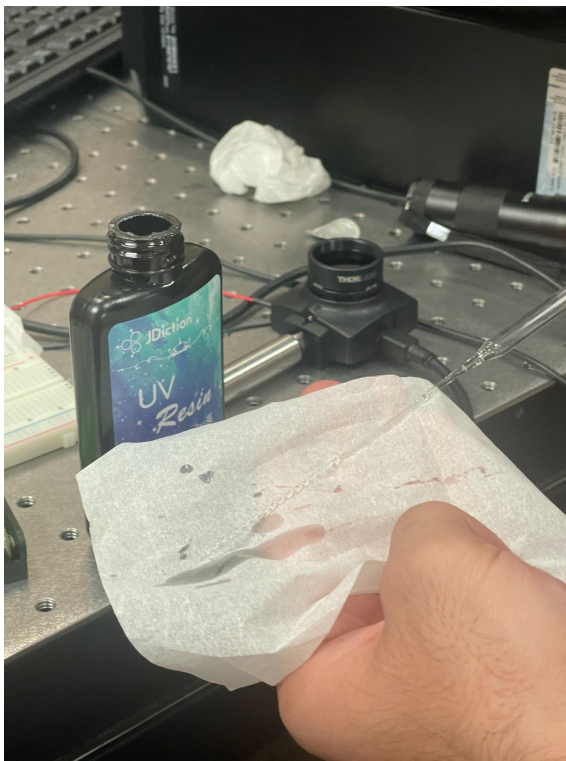
Figure 6.1-3. UV Resin being used to secure fiber to LED after coupling.
