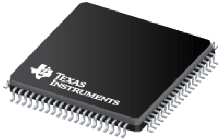
Figure 4.2.12-1. Example of a MSP430F5519
