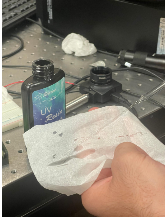
Figure 3.3.4-1. UV Resin To Seal LED-Fiber Coupling
